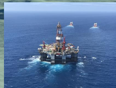
Ocean Monarch at Casino 5 Sole Drill Centre Water Depth - 125m Two Horizontal "Christmas" Tree Drill Depth - 2 x 1200m Drilling Length - 2,150m
