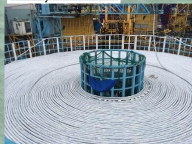
Umbilical spooling, UK. Umbilical 70% complete
